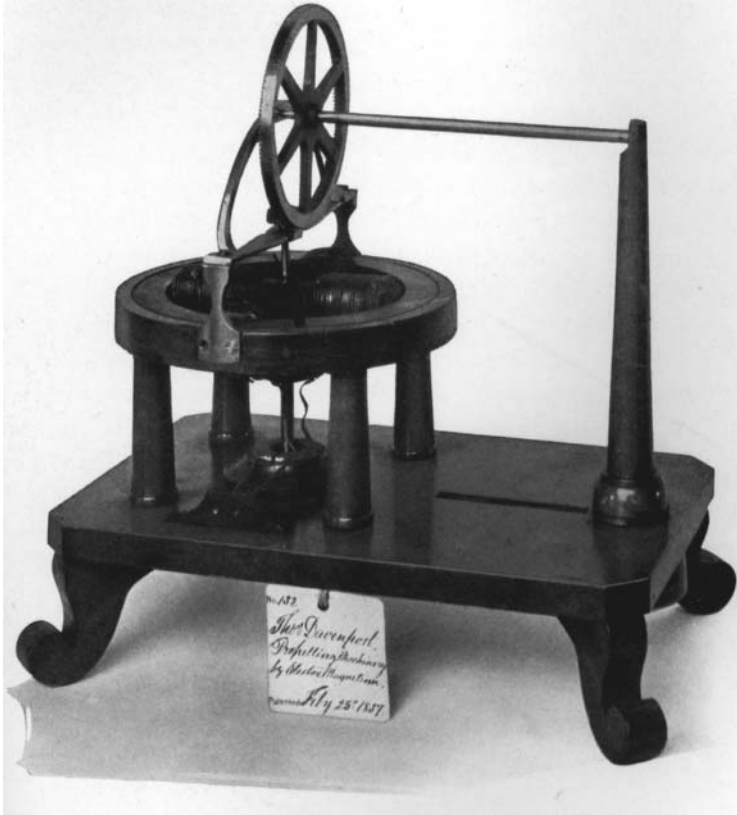
FIGURE 1.4 Thomas Davenport's electric motor, patented in 1837 (from Davenport 1929). Reprinted by permission of the Vermont Historical Society.
